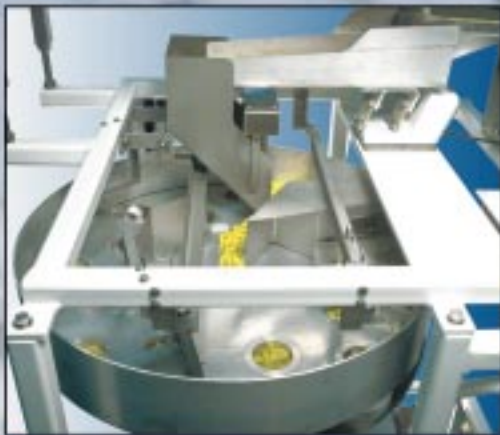
Product is distributed into the revolving head where cups are evenly filled prior to discharge.
